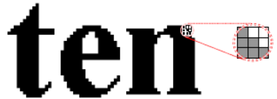
Fig 2: Illustration of a boundary pixel in the magnified view on some portion of the ‘n’ character
